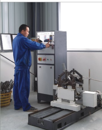
风叶动平衡试验 Leaf of the fan dynamic balancing testing
