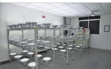
灯具老化试验 Lamp and Lanterns aging test room
